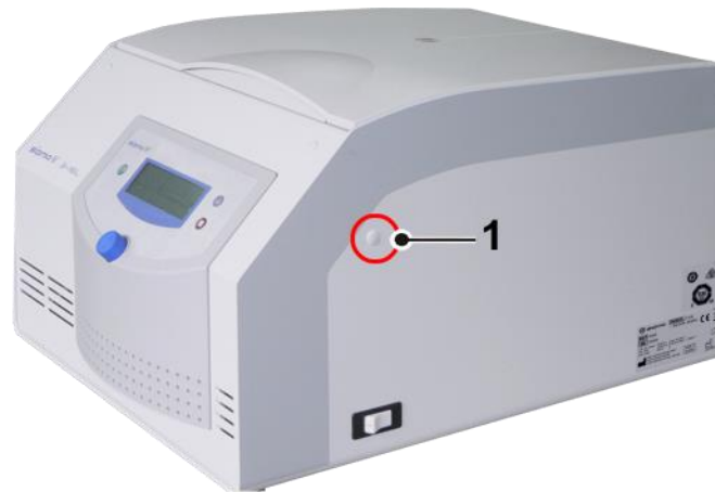
Fig. 31: Position of the opening for the emergency lid release
