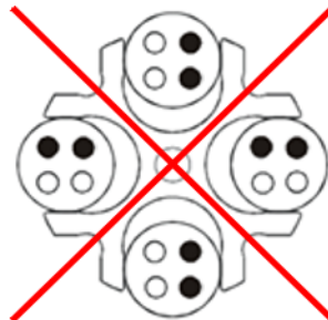
Fig. 12: Permissible and impermissible loading of an angle rotor and a swing-out rotor (example illustrations)
