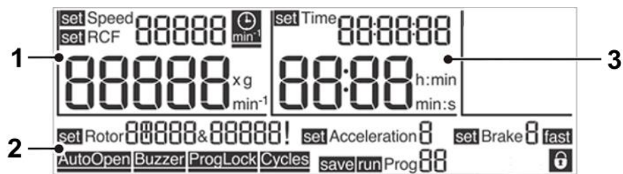
Fig. 15: Display of the "Spincontrol L" control system
